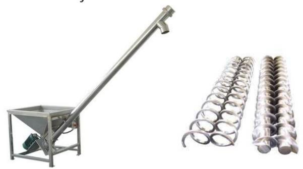
Drehen's Flexible Conveyors are based on latest technology support so as to provide optimum functional values in given operation areas. A flexible screw conveyor can outperform rigid screw conveyors, bucket elevators, chain conveyors, and other equipment intended to transport dry bulk solids. Flexible Screw Conveyor uses single moving part to convey material in any direction whether it be horizontal, vertical or routed around. These conveyors can be elevated as high as to 60 degrees.
